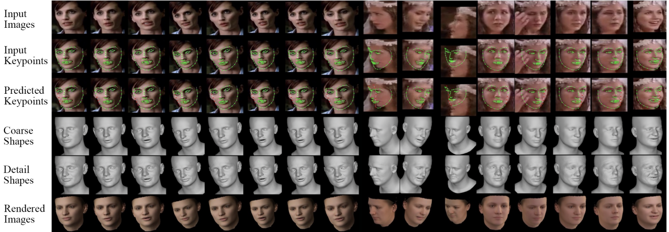
Figure 3: DECA results on Castle and Friends sequences trained with our dataset. Red points in predicted keypoints are the ones predicted incorrectly.
